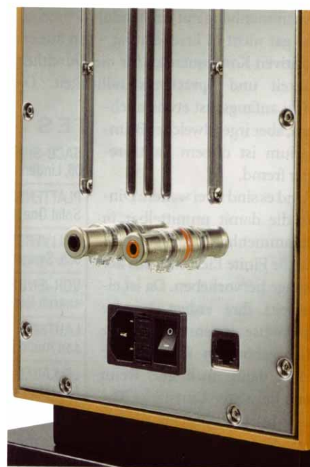
WBT polarity clamps for the external amplifier, mains connections to supply the integrated bass amp and socket for the remote control (r.)
